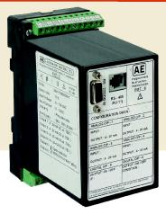
The PMT-9 Multifunction Programmable Transducer measures the several variables of an electric power system and process them to produce 4 analog output signals. 2 digital output signals are available for signaling the limits or energy metering pulses. The limits of the outputs can be set by individual measurand or logically combine up to three measurands.
